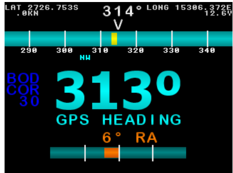
Figure 20: Example GPS Steer Mode Main Screen. Live Compass heading is 314°, Target Heading is 313°, Deviation is shown as a yellow bar within the compass bar.
