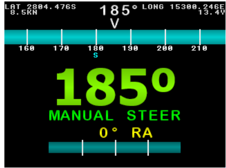
Figure 18: Example Manual Steer Mode Main Screen. Live Compass heading is 185°, Rudder is at center.
